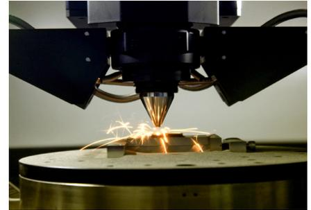
Gas requirements differ based on the process and the material being printed. For example, a direct metal laser sintering machine printing with cobalt chrome may require nitrogen, while a selective laser melting machine using the same material may require argon. Table II illustrates recommended gases for commonly used metal powders and printing technologies.
