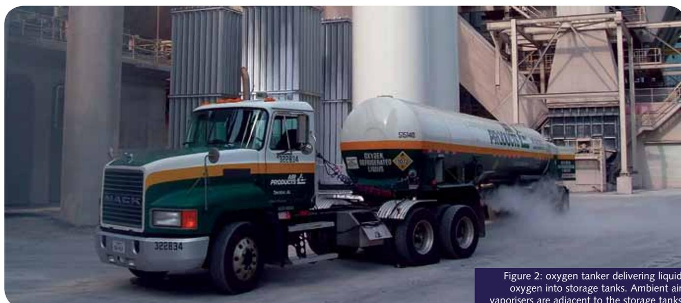
Figure 2: oxygen tanker delivering liquid oxygen into storage tanks. Ambient air vaporisers are adjacent to the storage tanks
